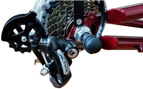
Fit the rear derailleur on the rear dropout.
