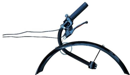
Fit the handlebars on the king post, tighten the bolt and fit headset cover.
