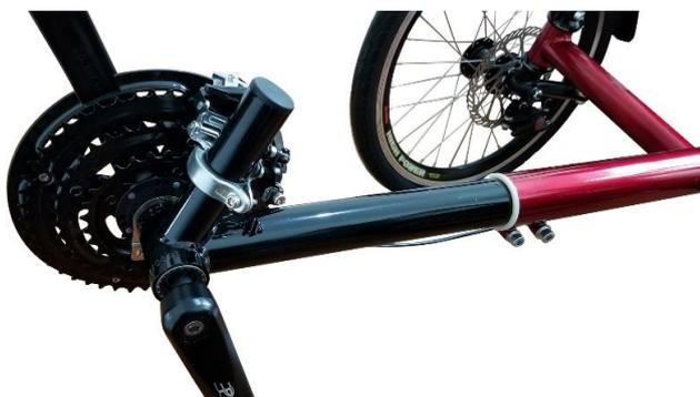
Carefully slide the boom into the beam. Take care not to damage the frame shim located inside the frame. Adjust the boom by twisting and pushing or pulling. Fasten the boom by the bolts under the beam.
