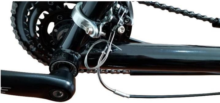
Pass the front derailleur cable through the cable guide hole under the beam. While holding the cable taut, turn the shifter through its range of movement to check the cables moves smoothly and that the cable is properly seating inside the shifter.
