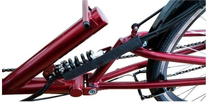
Check that the cable does not foul the seat or the track rod anywhere within the full range of steering movement.
