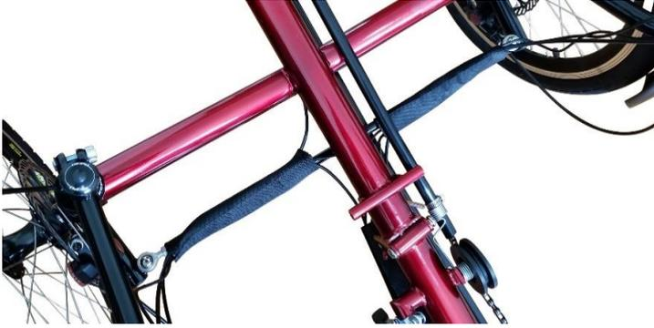
Fasten the cables on the track rod with the Velc
